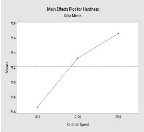
Fig.7. Main Effects Plot for Hardness Vs Rotation Speed
