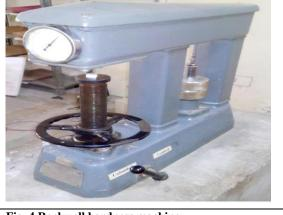
Fig. 4 Rockwell hardness machine
